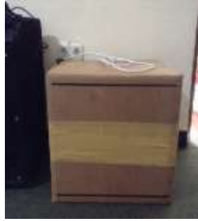
Figure 2. Yoghurt fermentation process (a) Sterile Bottle Contained a Milk Mixture and Yoghurt Starter ready fermented in an incubator of 37°C-45°C for 2x24 hours, (b) Artificial incubator made from cardboard with a temperature of 37°C-45°C
