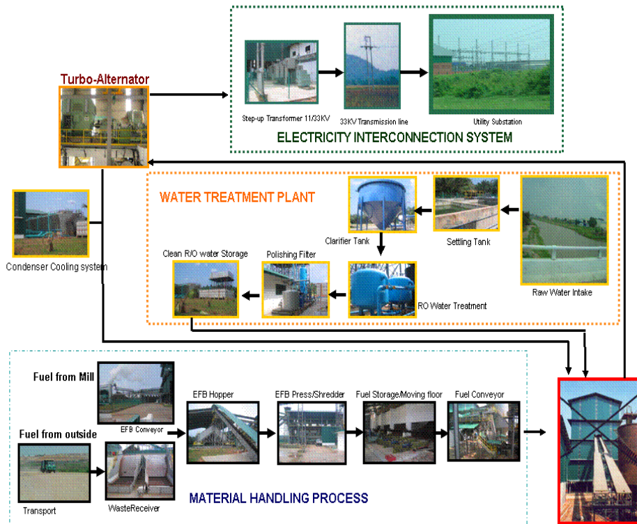
Picture 1 Alternative Biomass Power Plant
