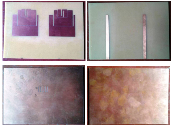
Fig. 4. Realized array antenna; two antenna elements on top side of first layer (top-left); microstrip feeding line on top side of second layer (top-right); groundplane with U-shaped DGS on bottom side of second layer (bottom-left); groundplane without U-shaped DGS on bottom side of second layer (bottom-right).
