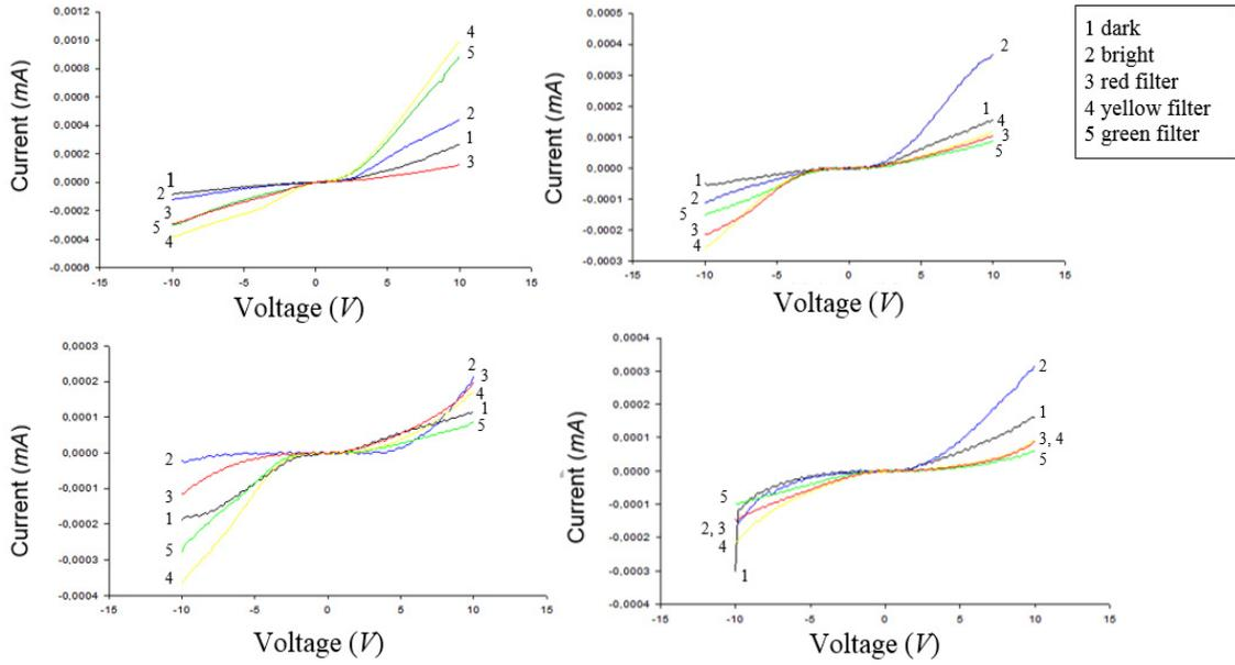
Fig. 1. I-V characteristic of BST with annealing time of (a) 8 hours; (b) 15 hours; (c) 22 hours; (d) 29 hours
