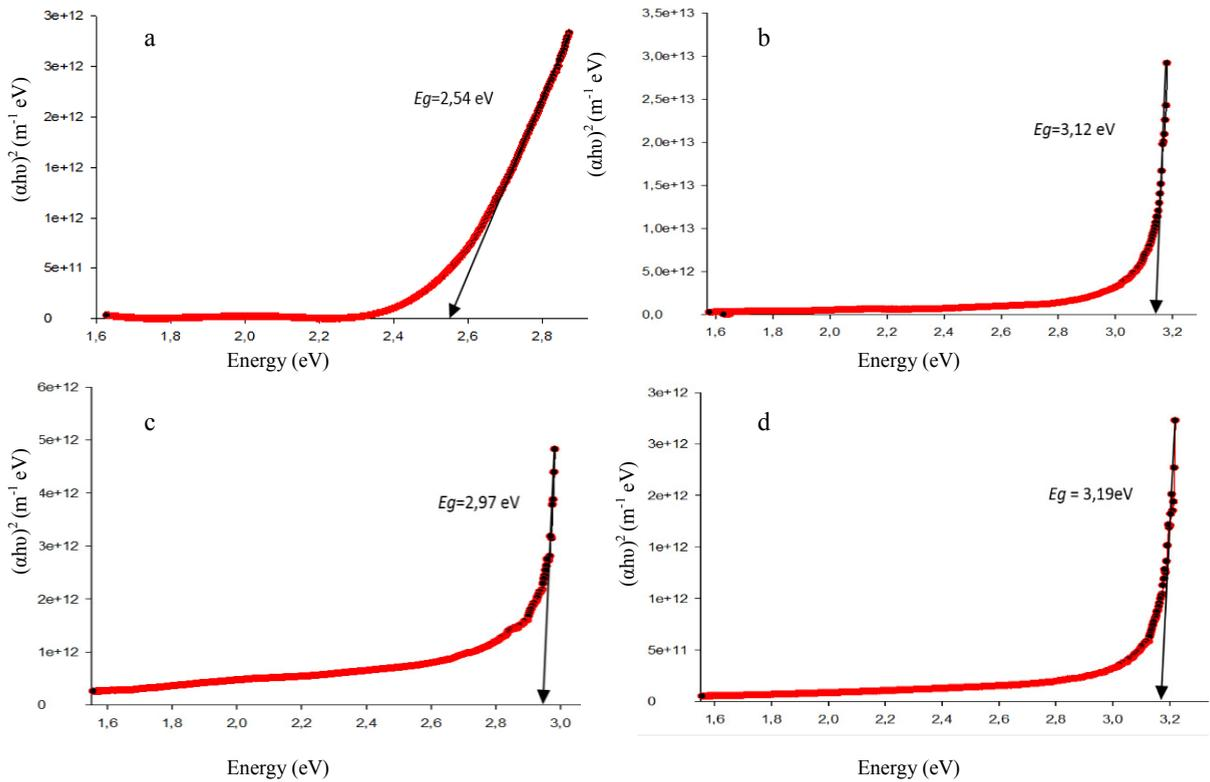
Fig. 3. Band gap energy determination using reflectance spectrum of BST with annealing time of (a) 8 hours; (b) 15 hours; (c) 22 hours; (d) 29 hours
