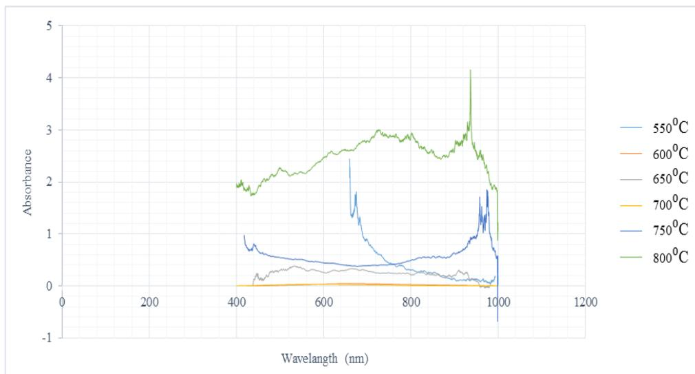
Fig. 2 Absorbance relations and wavelength LiTaO<sub>3</sub> film after the annealing process
