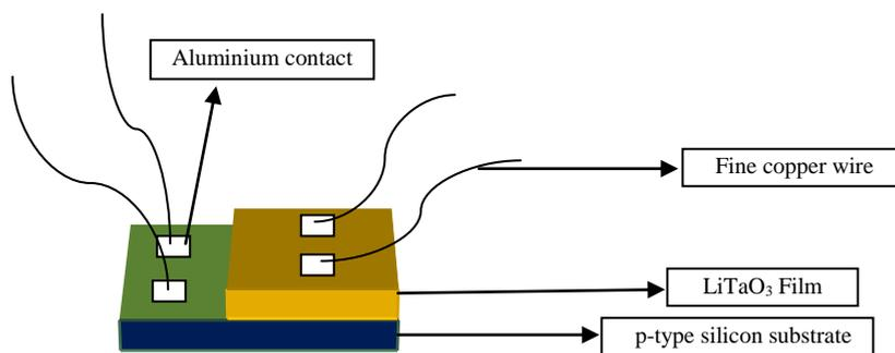
Fig. 1 Design of  $\text{LiTaO}_3$  ferroelectric
