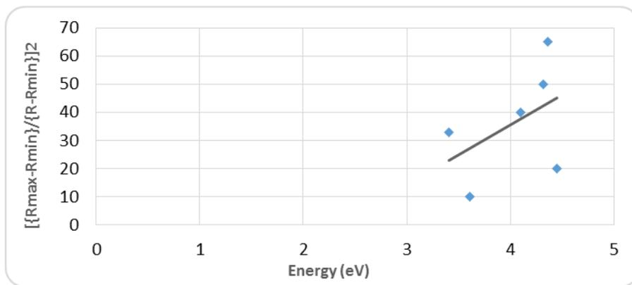
Fig. 4 Energy band-gap film LiTaO<sub>3</sub> after the process of annealing
