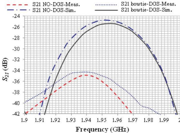
Fig. 5. Measurement and simulation results of  $S_{21}$  for array antenna with and without bowtie-shaped DGS.
