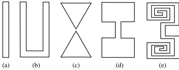
Fig. 1. Some types of DGS; (a) rectangular slot; (b) U-shaped slot; (c) bowtie-shaped slot; (d) square-slot dumbbell; (e) spiral-head dumbbell.
