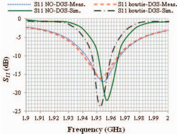
Fig. 4. Measurement and simulation results of  $S_{11}$  for array antenna with and without bowtie-shaped DGS.
