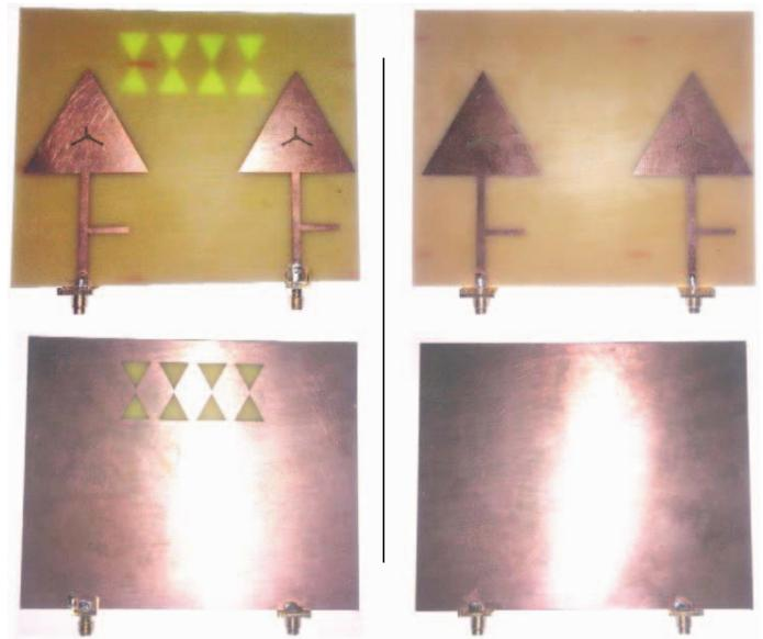
Fig. 3. Fabricated planar array antenna; left is with bowtie-shaped DGS (top-bottom); right is without DGS (top-bottom).
