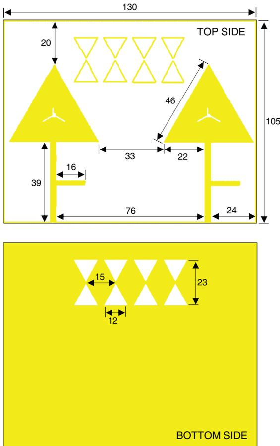
Fig. 2. Construction of proposed planar array antenna with bowtie-shaped DGS (unit in mm).
