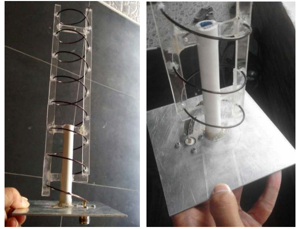
Fig. 3. Realized monofilar helical antenna standing on an aluminium metal.
