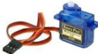
*Figure 2. Motor Servo*
